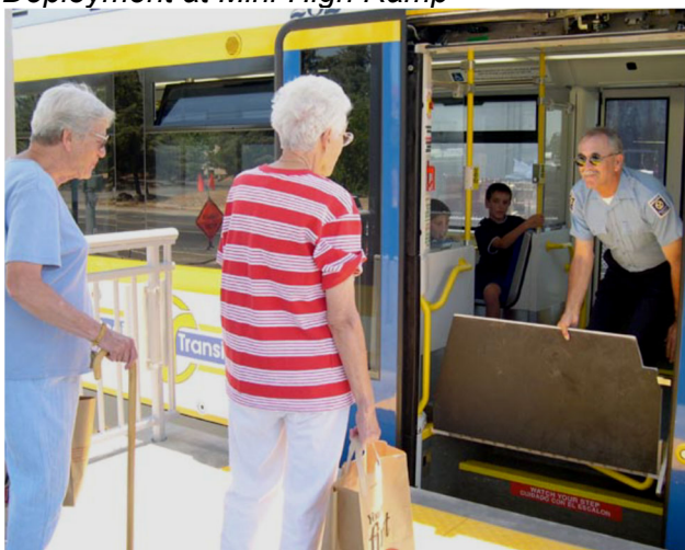
Figure 29: Bridge Plate Deployment at Mini-High Ramp
