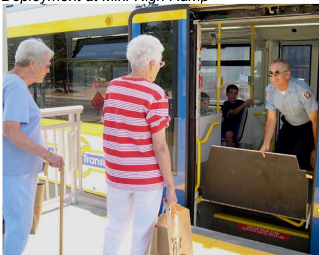
Figure 29: Bridge Plate Deployment at Mini-High Ramp
